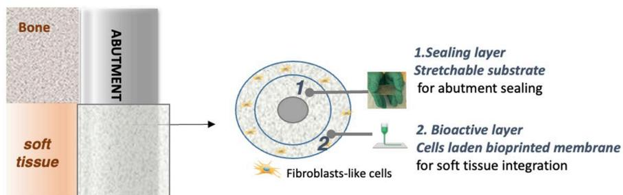
*Fig. 2 - Schematic representation of a bilayer scaffold.*
