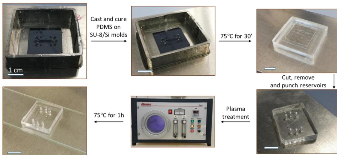
Fig. 6. Schematic of the different steps for the fabrication of PDMS microfluidic devices.
