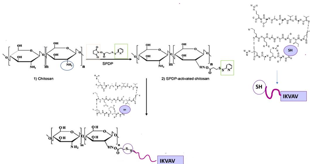
Fig. 3 Reaction mechanism of Chitosan functionalization with the IKVAV small peptide motif.
