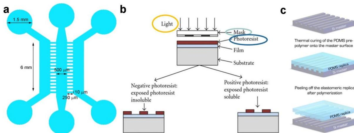
**Fig. 5.** Schematic of a preliminary 3-unit microfluidic device (a), fabricated by photolithography (b) and soft lithography (c) approaches.
