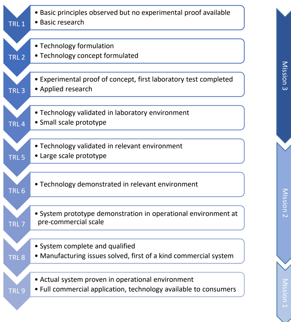
Fig. 1 Technology Readiness Levels, as described and used by the European Commission, and how they are reflected in the three Fit4Med Missions.
