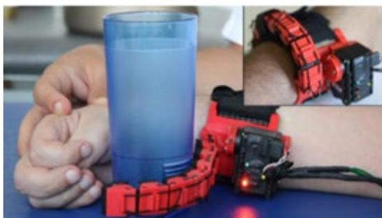
*Figure 1 - Sixth finger developed at UNISI.*
