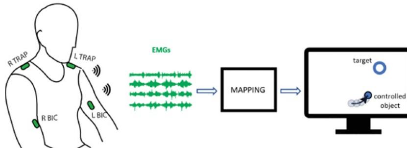
Fig. 13 - Cursor movement controlled by biceps muscles.
