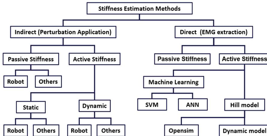
Fig. 2 - Classification of the Stiffness Estimation Method.
